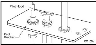
Fig. 59 Remove pilot hood.
